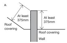
The wall should be extended up through the roof for a height of at least 375mm above the top surface of the adjoining roof covering.
