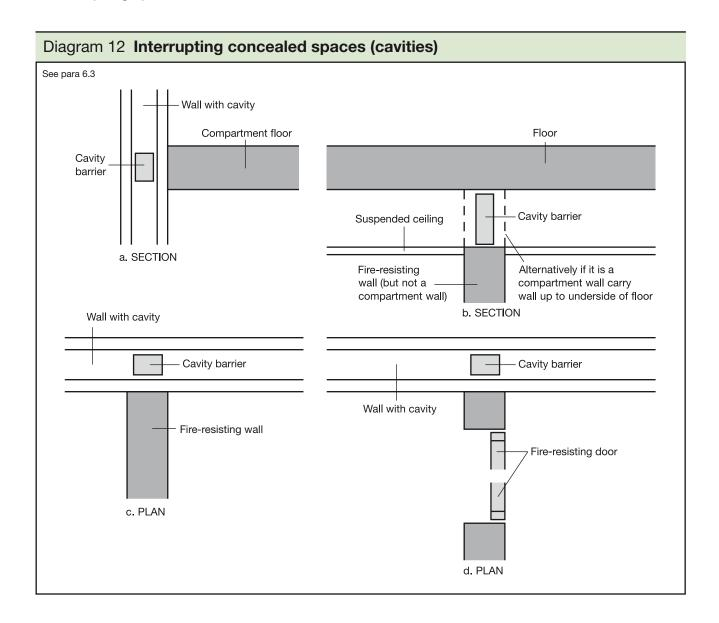
It is important to continue any compartment wall up through a ceiling or roof cavity to maintain the standard of fire resistance – therefore compartment walls should be carried up to the roof, see paragraph 5.11. It is not appropriate to complete a line of compartment walls by fitting cavity barriers above them.
