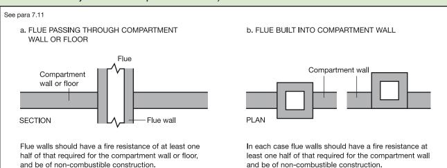
7.11 If a flue or duct containing flues or appliance ventilation duct(s), passes through a compartment wall or compartment floor, or is built into a compartment wall, each wall of the flue or duct should have a fire resistance of at least half that of the wall or floor in order to prevent the by-passing of the compartmentation (see Diagram 16).
